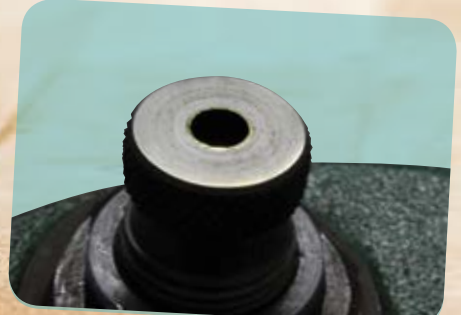
Excessive case length that was filed flat.
