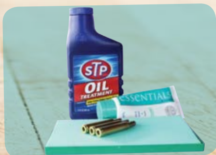
Good lubrication is essential when processing cases through the decapping and sizing die.
