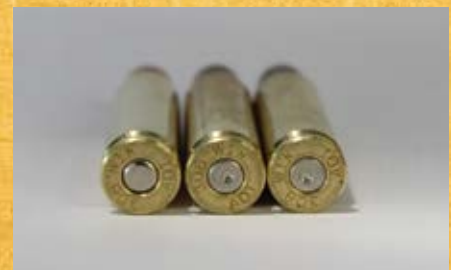
Note progressive primer flattening.
