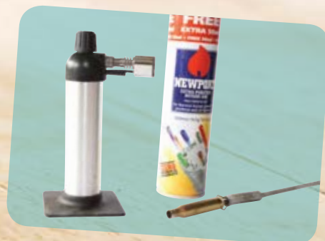
Annealing can be done with minimum tools.
