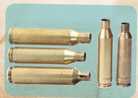
Split necks and partial case separation.
